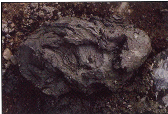
Figure 6. Piece of gray clay confining layer material removed during the installation of the 24-inch diameter well casing for the Tolan Farm well.
