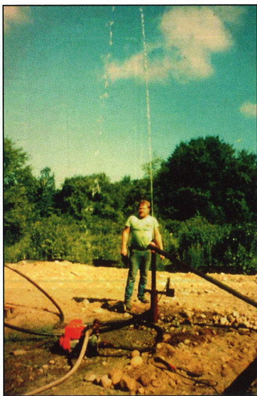
Figure 3. Water squirting into the air to a height of approximately 26 feet above ground surface caused by the hydraulic head in the confined aquifer.
