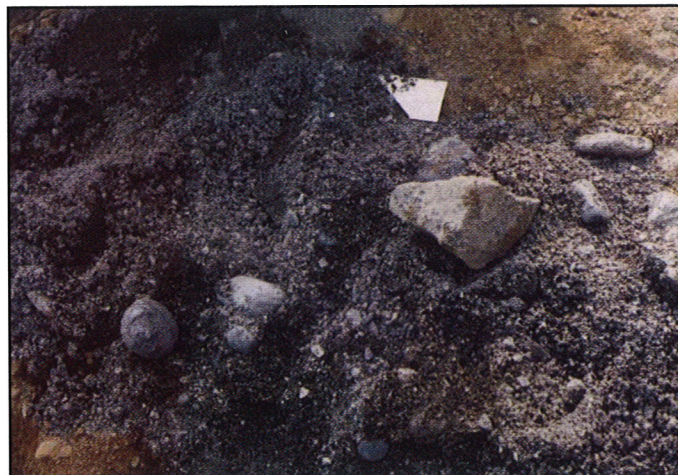
Figure 8. Close-up of aquifer material from the well screen area of the Tolan Farm well. Size of cobbles are up to 6-inches.
