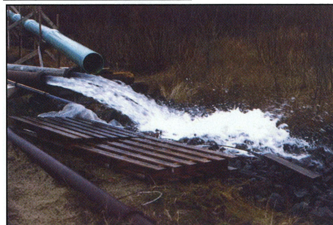
Figure 5. (below) Tolan Farm well pumping test discharge of 1,560 gallons per minute during the 5-day aquifer pumping test.
