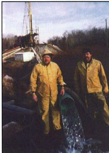
Figure 4. “Free flow” discharge from the Tolan Farm well. Free flow rate is approximately 1,000 gallons per minute. The discharge line from the well is 12-inches in diameter.
