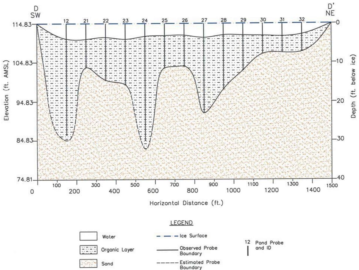
**FIGURE 6.** Geologic Cross-Section D-D' of On-Site Pond, Brewster Wellfield.
