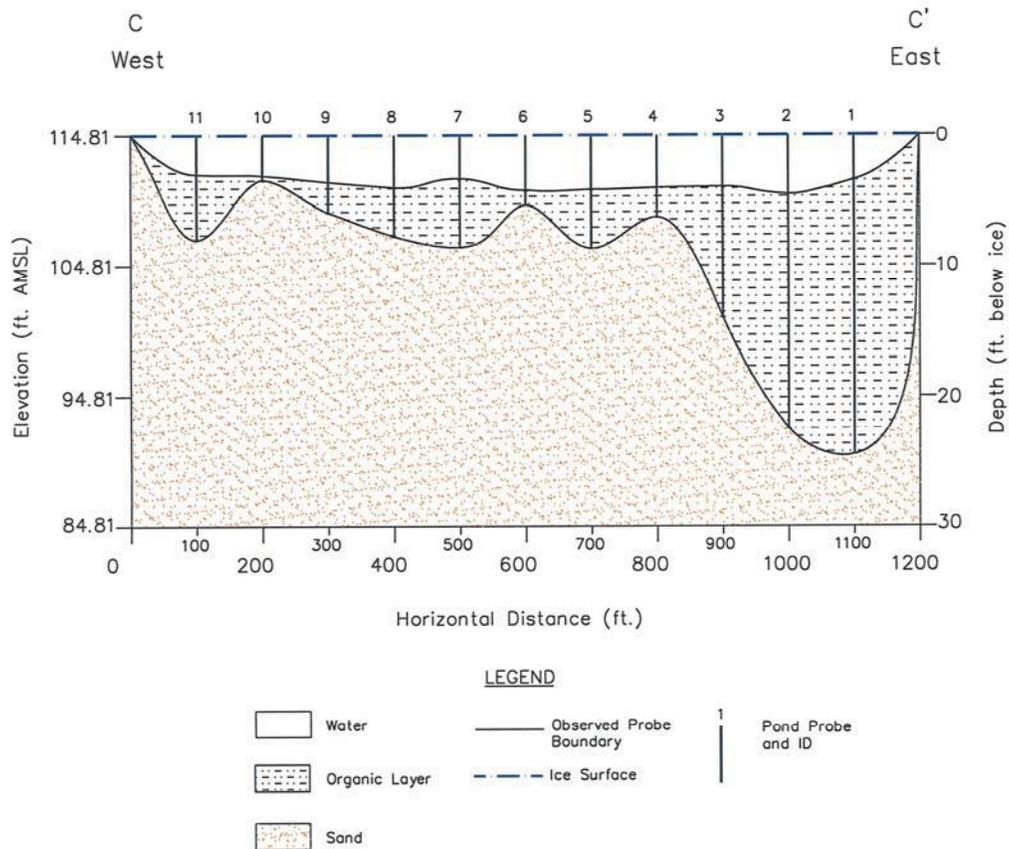
**FIGURE 5.** Geologic Cross-Section C-C' of On-Site Pond, Brewster Wellfield.
