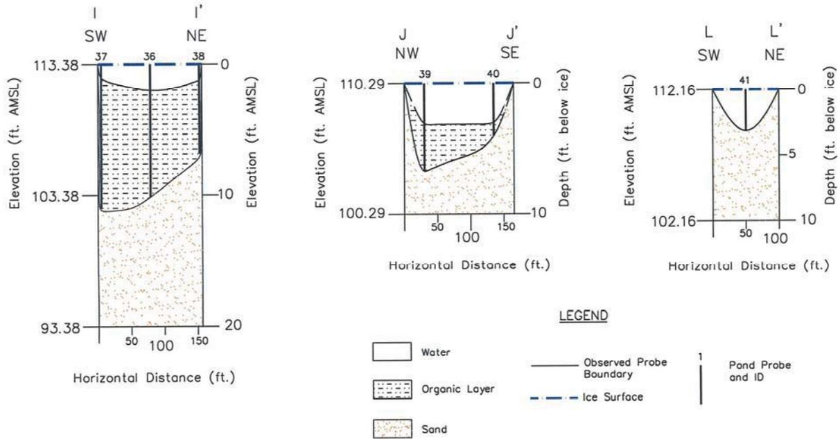
**FIGURE 7.** Geologic Cross-Sections I-I', J-J', and L-L' of On-Site Kettle Hole Ponds, Brewster Wellfield.
