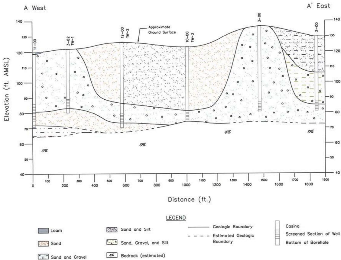
Figure 3. Geologic Cross-Section A-A', Brewster Wellfield.
